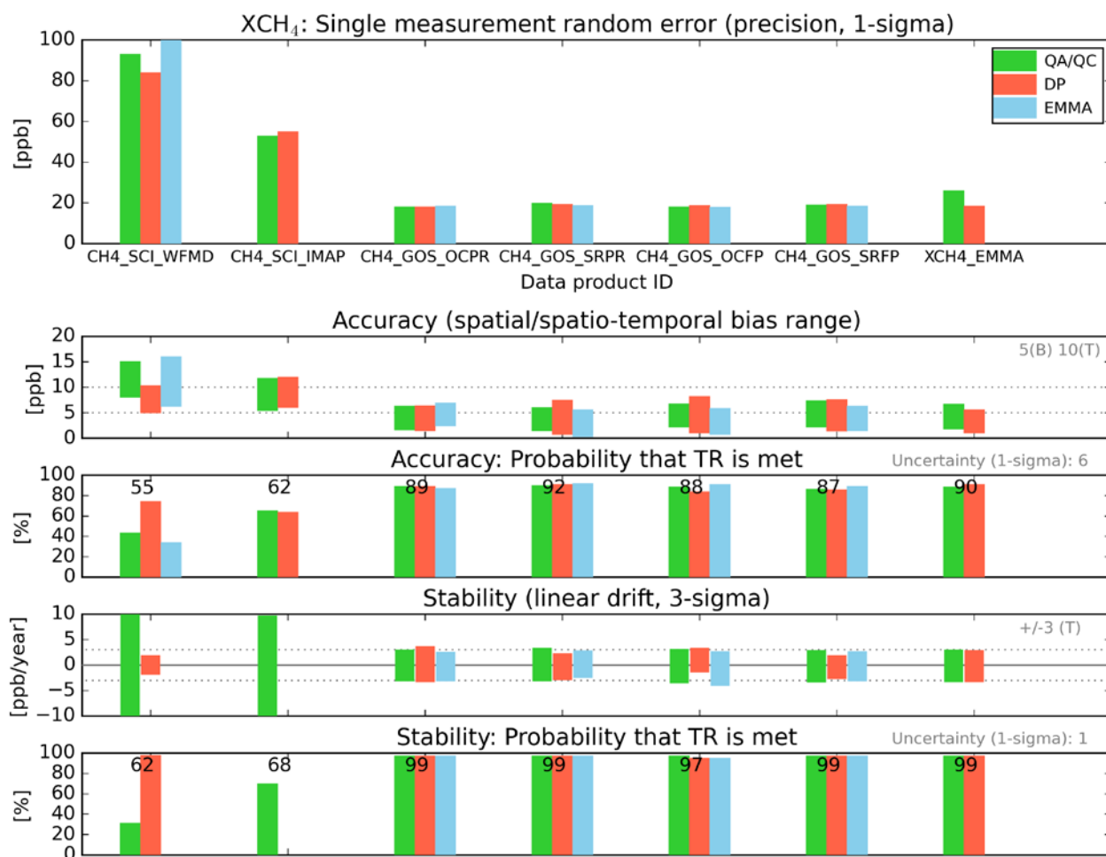
Figure 37 - Overview data quality assessment results for Level 2 XCH 4 data products. The green bars refer to the “Quality Assessment / Quality control” (QA/QC) results as described in this document. The red bars refer to results obtained by the data providers (DPs), as described in separate Annexes (see Sect. 9). For “Accuracy” and “Stability” also the numerical values for the “Probability that TR is met” are given (computed as mean value if more than one value (bar) exists). Also listed (in grey on the right hand side) is the uncertainty of the reference data as used for the Target Requirement (TR) assessments.
